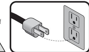
**WARNING** When using an extension cable, verify the gauge is enough for the power that your product needs. A lower gauge cable will cause voltage drop in the line, resulting in power loss and overheating. The following table shows the right size to use depending on cable's length and the ampere capability shown in the tool's nameplate. When in doubt use the next higher gauge.
